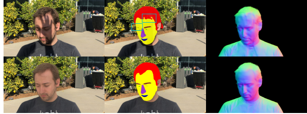
Figure 12. Light diffusion (bottom left) can improve results of state-of-the-art image processing methods, such as face parsing [16] (middle, improvement in green boxes) or normal map estimation (right, removal of shadow embossing).
