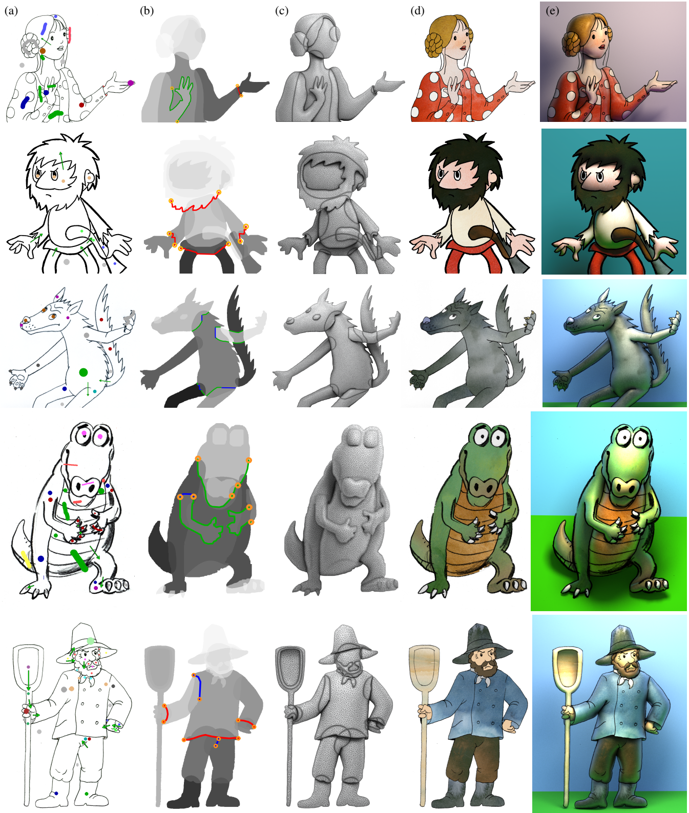
Fig. 26. Results—(a) the original drawing including user-defined annotations for segmentation, (b) result of the layering and completion phase with boundary condition annotations (red: Neumann and C^\infty , green: Dirichlet and C^\infty , blue: Neumann and C^1 grafting), (c) generated bas-relief-type mesh, (d) original texture, (e) resulting global illumination render. (Source drawings: lady, wolf, dino, and farmer © Anifilm, robber © UPP. All rights reserved.)
