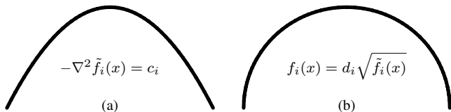
Fig. 10. Shape profiles—(a) initial parabolic profile produced by the Poisson equation, (b) spherical profile obtained by applying a cross-section function with square root.
